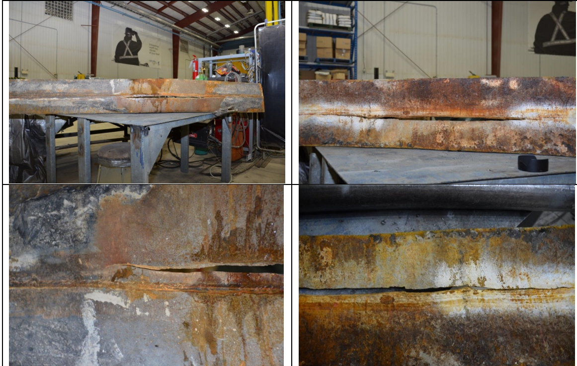
Figure 4-1: Close-up View of the Rupture in Can 35 (in the Laboratory for Material Tests)
