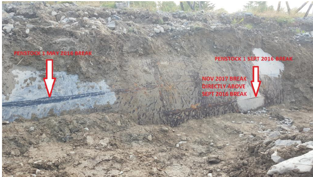
Figure 2: Rupture locations on Penstock 1 Bay d'Espoir
